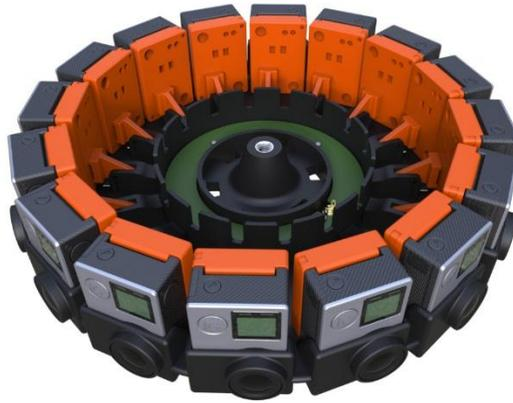
*Google's Jump 16-camera rig (there are other competitive devices) simultaneously captures 360 degree scenery. Images from each camera can be stitched together to create dynamic backgrounds for virtual and augmented reality systems.*
